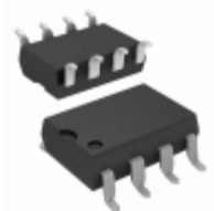
6N139S(TA)-V Everlight Electronics Co Ltd OPTOISO 5KV DARL W/BASE 8SMD
