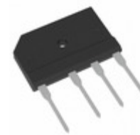
TS15P05G D2G TSC (Taiwan Semiconductor) BRIDGE RECT 1P 600V 15A TS-6P
