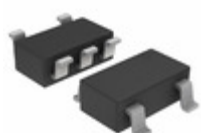
NCP500SN33T1 ON Semiconductor IC REG LDO 3.3V 0.15A 5TSOP
