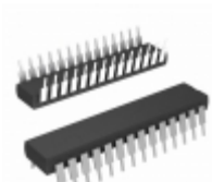
PIC16C73B-04/SP Microchip Technology IC MCU 8BIT 7KB OTP 28SDIP
