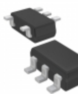
XC6121D529MR-G Torex Semiconductor Ltd IC WATCHDOG TIMER SOT-25
