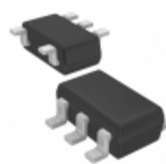
XC6121D532MR-G Torex Semiconductor Ltd IC WATCHDOG TIMER SOT-25
