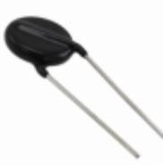
ERZ-E14A431 Panasonic Electronic Components VARISTOR 430V 10KA DISC 16.5MM
