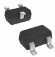
DDTC122LE-7-F Diodes Incorporated TRANS PREBIAS NPN 150MW SOT523
