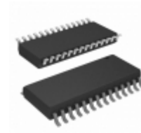
AT28HC64B-70SI Microchip Technology IC EEPROM 64KBIT 70NS 28SOIC
