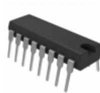
MC10H136PG ON Semiconductor IC COUNTER UNIV HEX HS 16-CDIP
