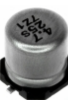
ECE-V1EA4R7NR Panasonic Electronic Components CAP ALUM 4.7UF 20% 25V SMD
