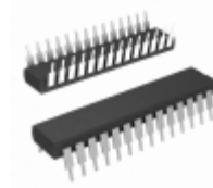
DSPIC33EP32MC502-I/SP Microchip Technology IC MCU 16BIT 32KB FLASH 28SDIP
