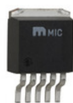
MIC29152BU Microchip Technology IC REG LDO ADJ 1.5A TO263-5
