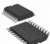
PIC16C58B-04E/SO Microchip Technology IC MCU 8BIT 3KB OTP 18SOIC
