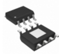
ADP7105ARDZ-1.8 Analog Devices Inc. IC REG LDO 1.8V 0.5A 8SOIC
