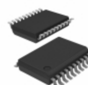
PIC16C621-20I/SS Microchip Technology IC MCU 8BIT 1.75KB OTP 20SSOP
