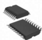
PIC16C621A-04I/SO Microchip Technology IC MCU 8BIT 1.75KB OTP 18SOIC
