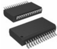
PIC16C57T-HS/SS Microchip Technology IC MCU 8BIT 3KB OTP 28SSOP
