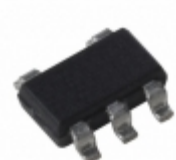
MIC5245-3.5BM5-TR Microchip Technology IC REG LDO 3.5V 0.15A SOT23-5
