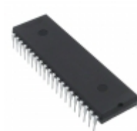
TS80C32X2-VIA Microchip Technology IC MCU 8BIT ROMLESS 40PDIL
