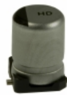
EEV-HD1HR47R Panasonic Electronic Components CAP ALUM 0.47UF 20% 50V SMD
