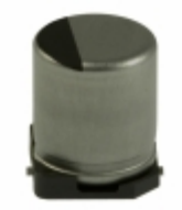
EEE-1AA221XP Panasonic Electronic Components CAP ALUM 220UF 20% 10V SMD
