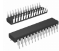
PIC18F2610-I/SP Microchip Technology IC MCU 8BIT 64KB FLASH 28SDIP
