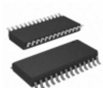
PIC18F2610T-I/SO Microchip Technology IC MCU 8BIT 64KB FLASH 28SOIC
