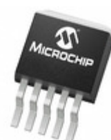
MCP1825-1202E/ET Microchip Technology IC REG LDO 1.2V 0.5A DDDPAK
