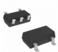
S-1112B24MC-L6JTFFU SII Semiconductor Corporation IC REG LINEAR 2.4V 0.15A SOT23-5
