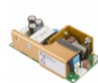
ECM60UT34 XP Power AC/DC CONVERTER 3.3V 5V 12V 60W
