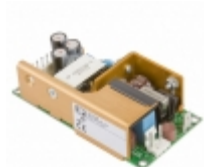
ECM60UT32 XP Power AC/DC CONVERTER 5V +/-12V 60W
