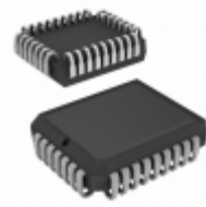
AT28C17-20JI Microchip Technology IC EEPROM 16KBIT 200NS 32PLCC
