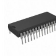
AT28C17-20PC Microchip Technology IC EEPROM 16KBIT 200NS 28DIP
