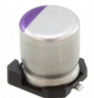
2R5SVPE330MY Panasonic Electronic Components CAP ALUM POLY 330UF 20% 2.5V SMD
