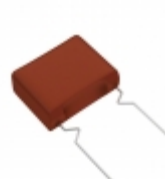
ECW-F2125HAQ Panasonic Electronic Components CAP FILM 1.2UF 3% 250VDC RADIAL
