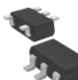
XC6121C544MR-G Torex Semiconductor Ltd IC WATCHDOG TIMER SOT-25
