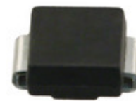
TVB090RSC-L Littelfuse Inc. THYRISTOR 90V 400A SMB
