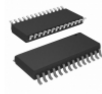
AD9708ARZRL Analog Devices Inc. IC DAC 8BIT 100MSPS 28-SOIC
