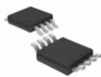
LT6657BHMS8-3#TRPBF ADI (Analog Devices, Inc.) IC VREF SERIES 3V 8MSOP
