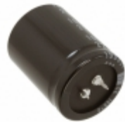
LAQ2D152MELC45 Nichicon CAP ALUM 1500UF 20% 200V SNAP
