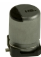
EEE-HB1C220AR Panasonic Electronic Components CAP ALUM 22UF 20% 16V SMD
