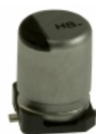
EEE-HB1C101AP Panasonic Electronic Components CAP ALUM 100UF 20% 16V SMD
