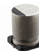
ULR2D220MNL1GS Nichicon CAP ALUM 22UF 20% 200V SMD
