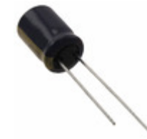
EEU-FC1C471LB Panasonic Electronic Components CAP ALUM 470UF 20% 16V RADIAL
