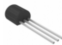
MN13811SLU Panasonic Electronic Components VOLT DETECT IC N-CH OD 3.0V TO92
