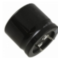
LGN2E821MELB35 Nichicon CAP ALUM 820UF 20% 250V SNAP
