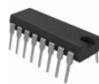
RE46C122E16F Microchip Technology IC SMOKE DETECTOR CMOS 16DIP
