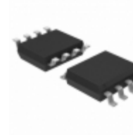
SST26WF080B-104I/SN Microchip Technology IC FLASH 8MBIT 104MHZ 8SOIC
