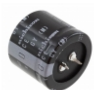
LGY1K332MELC30 Nichicon CAP ALUM 3300UF 20% 80V SNAP
