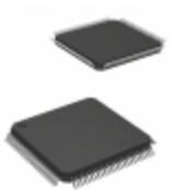
EFM32G880F64G-E-QFP100R Energy Micro (Silicon Labs) 64K FLASH, 16K RAM, 4X40 LCD, AE
