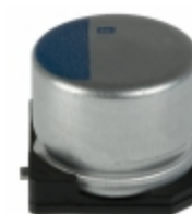
APXA2R5ARA681MHC0G United Chemi-Con CAP ALUM POLY 680UF 20% 2.5V SMD
