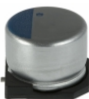
APXA4R0ARA122MJC0G United Chemi-Con CAP ALUM POLY 1200UF 20% 4V SMD
