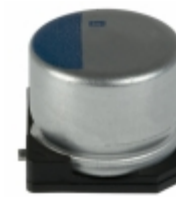
APXA4R0ARA221MH70G United Chemi-Con CAP ALUM POLY 220UF 20% 4V SMD
