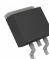
BA17807FP-E2 Rohm Semiconductor IC REG LDO 7V 1A TO252-3
