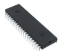
PIC16F914-I/P Microchip Technology IC MCU 8BIT 7KB FLASH 40DIP
