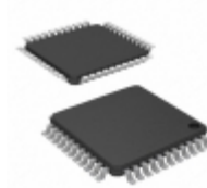
PIC16F914-I/PT Microchip Technology IC MCU 8BIT 7KB FLASH 44TQFP
