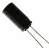
EEU-EB1H221 Panasonic Electronic Components CAP ALUM 220UF 20% 50V RADIAL
