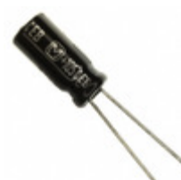
EEU-EB1H220SB Panasonic Electronic Components CAP ALUM 22UF 20% 50V RADIAL
