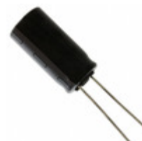
EEU-EB1H221B Panasonic Electronic Components CAP ALUM 220UF 20% 50V RADIAL
