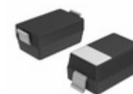
MMSZ6V8T3G ON Semiconductor DIODE ZENER 6.8V 500MW SOD123
