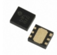
XC6124F616ER-G Torex Semiconductor Ltd IC WATCHDOG TIMER 6-USP
