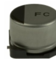
EEV-FC1C101P Panasonic Electronic Components CAP ALUM 100UF 20% 16V SMD
