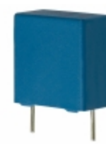
B32913A4473M289 EPCOS (TDK) CAP FILM 0.047UF 20% 440VAC RAD
