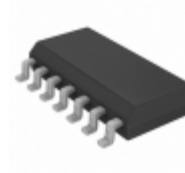
MCP4241T-502E/SL Microchip Technology IC DGTL POT 5K 2CH 14SOIC
